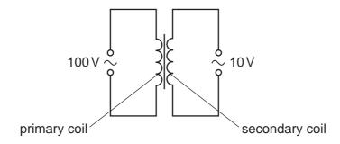
What are suitable numbers of turns for the primary coil and for the secondary coil?
