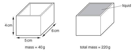
The box has a mass of 40 g when empty. When filled with a liquid, it has a total mass of 220 g.
